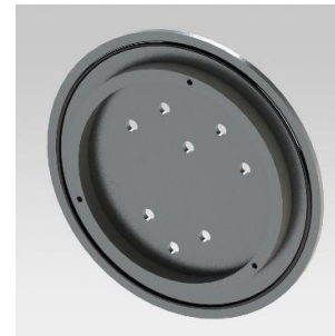
Figure 4. Rear end cap with O-ring groove
