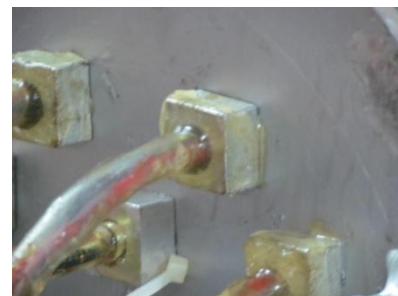
Figure 5. Penetrators on end cap
