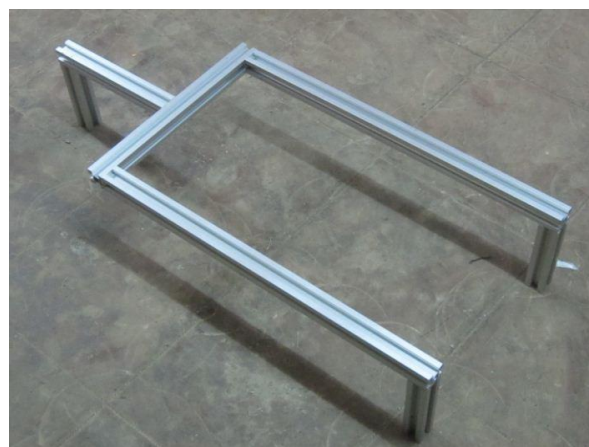
Figure 9. Skeletal structure of Matsya's frame
